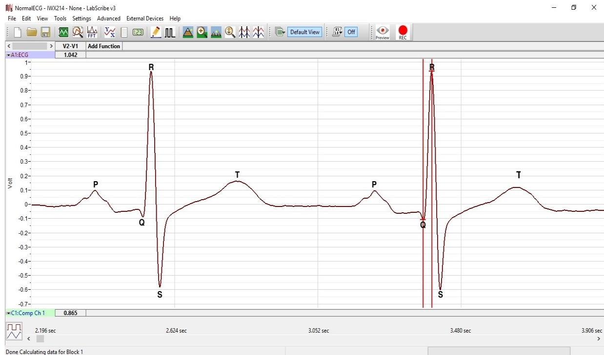
Figure HH-9-L3: ECG recording displayed in the Analysis window. Lines and labels were added to indicate the locations where cursors should be placed to measure the amplitudes of R (Q-R), P (Baseline-P), T (Baseline-T) waves; and, the length of the beat to beat period (R-R).
